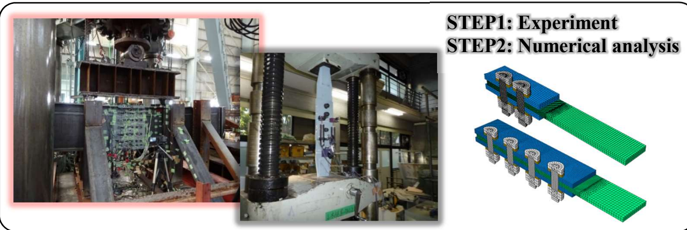
Fig. 2 Flow of this study to clarify the relationship among structural configurations, bearing resistance, ductility of joint
